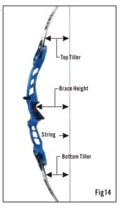
Typically, for most shooters with normal finger and hand pressure, anywhere from 0 to 3/8" of tiller is going to yield a bow which aims easily without "pulling" high or low, and which shoots more quietly.
