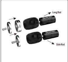
First tighten and fix the V-bar and the extender together, then screw the 5/16-24UNF screw at the other end of the side rod into the quick connector, align it with the round hole on the V bar, insert and tighten it to ensure firmness. The 5/16-24UNF screw at the other end of the long rod shall be directly tightened with the screw hole on the connector to ensure firmness.
